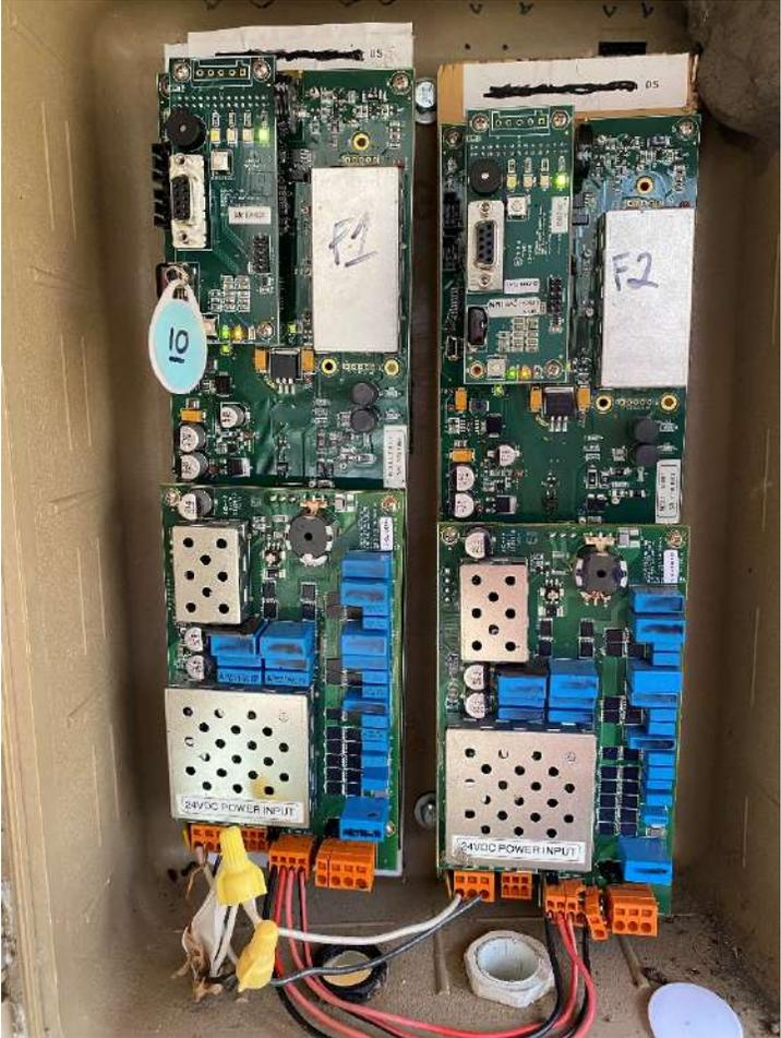
Picture 7. IS001 readers at French Creek downstream array.
