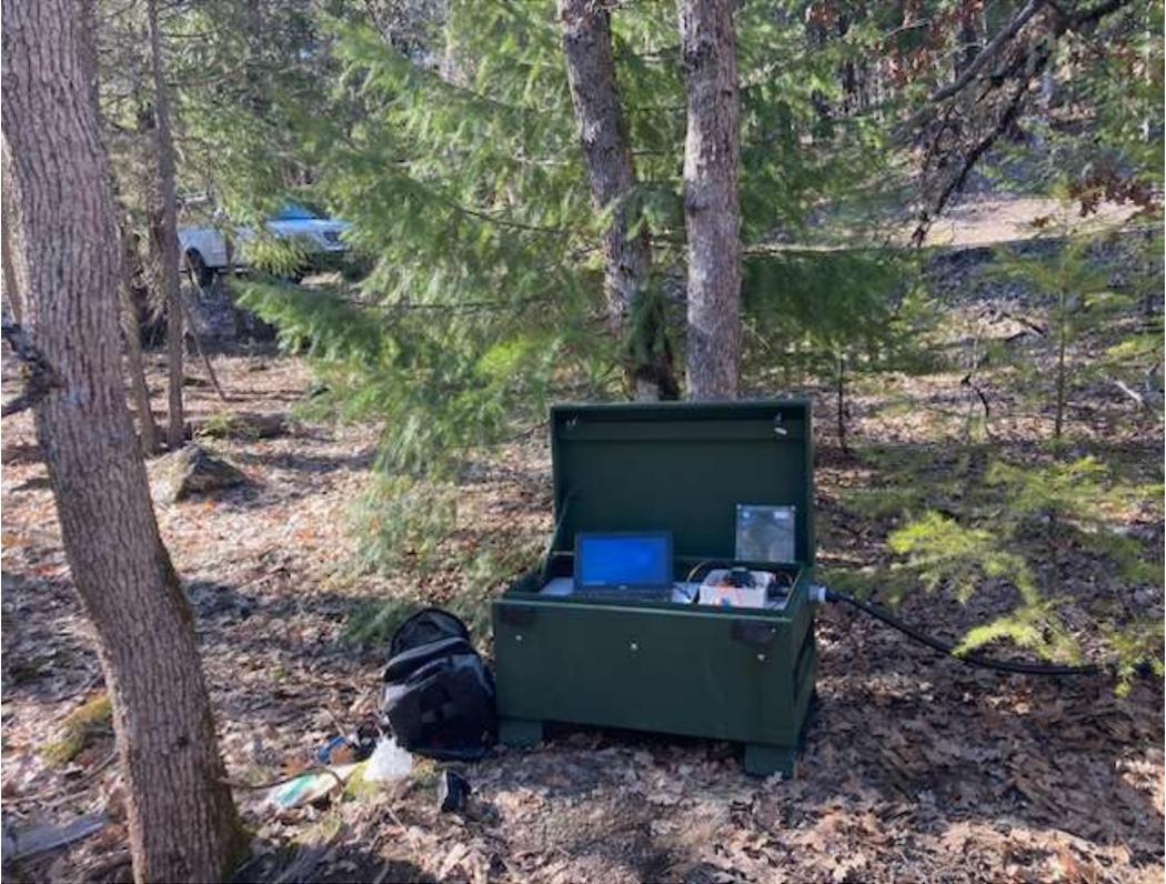
Picture 4. Data logger and power station at Scott River weir array.
