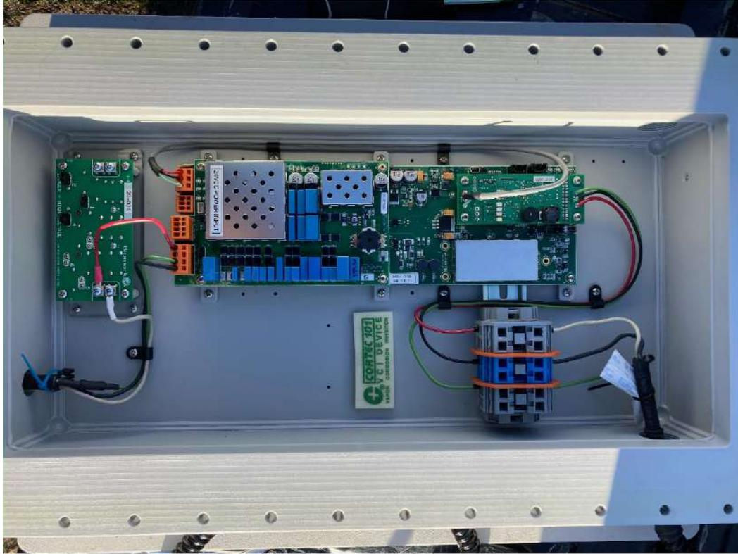
Picture 3. Fishway enclosure housing IS1001 reader and capacitance board.
