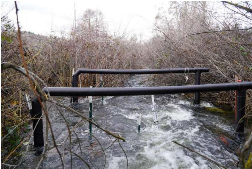
*Picture 10. Paired antennas at the Sugar Creek downstream array site.*
