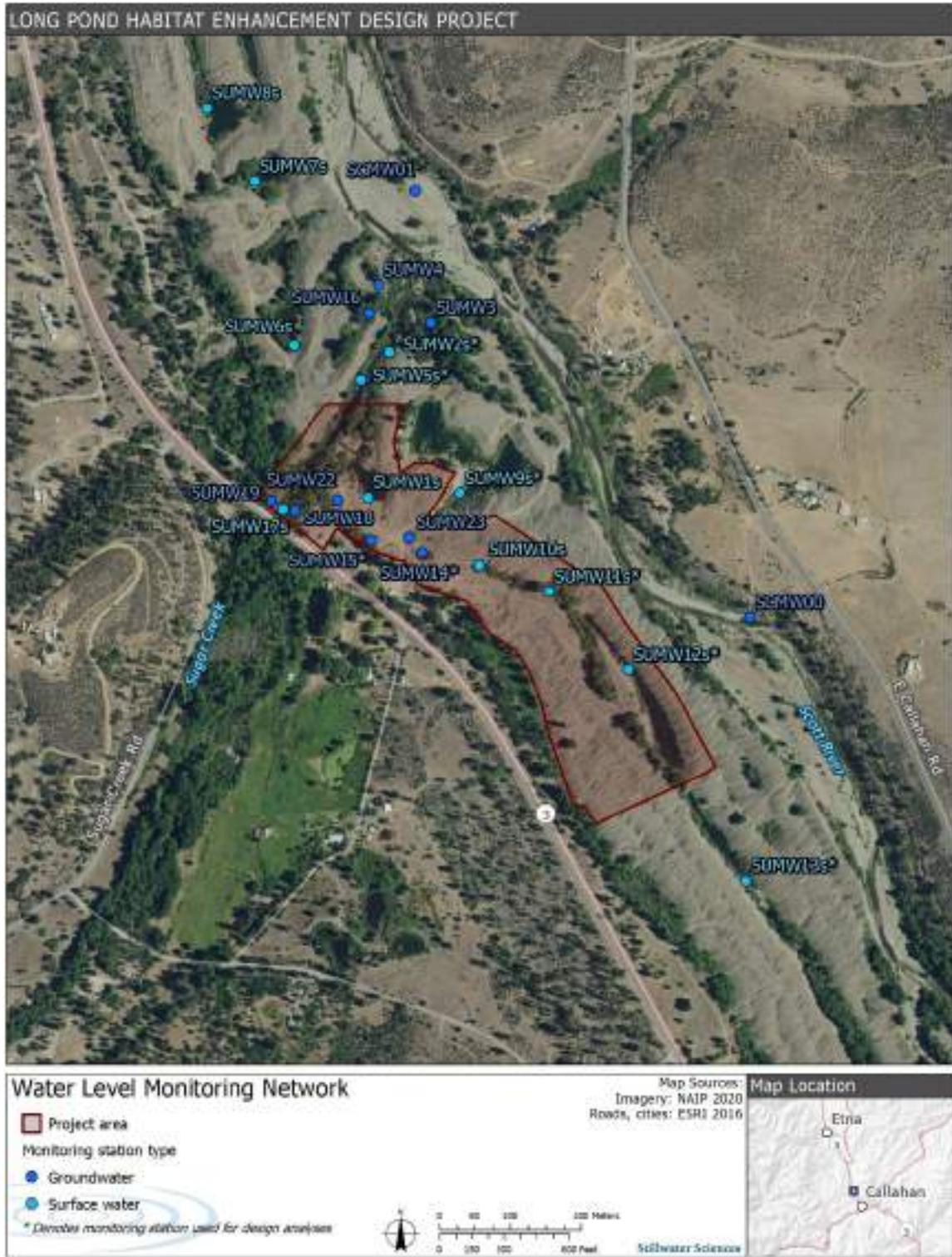
Figure 3-1. Surface water and shallow groundwater monitoring locations in the Project vicinity.
