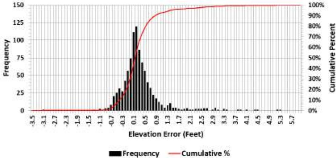
Figure 2-4. Histogram and cumulative distribution of elevation error between the initial DTM and selected survey points.
