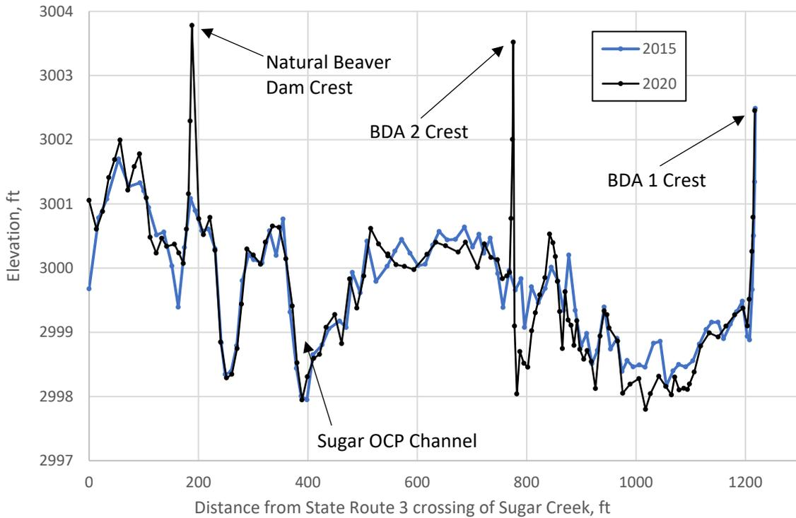
Figure H-3. Sugar Creek Longitudinal thalweg profile surveys in 2015 and 2020.
