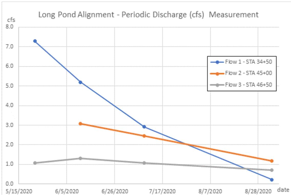
Figure 1 – Periodic discharge (cfs) measurements – Long Pond Alignment
