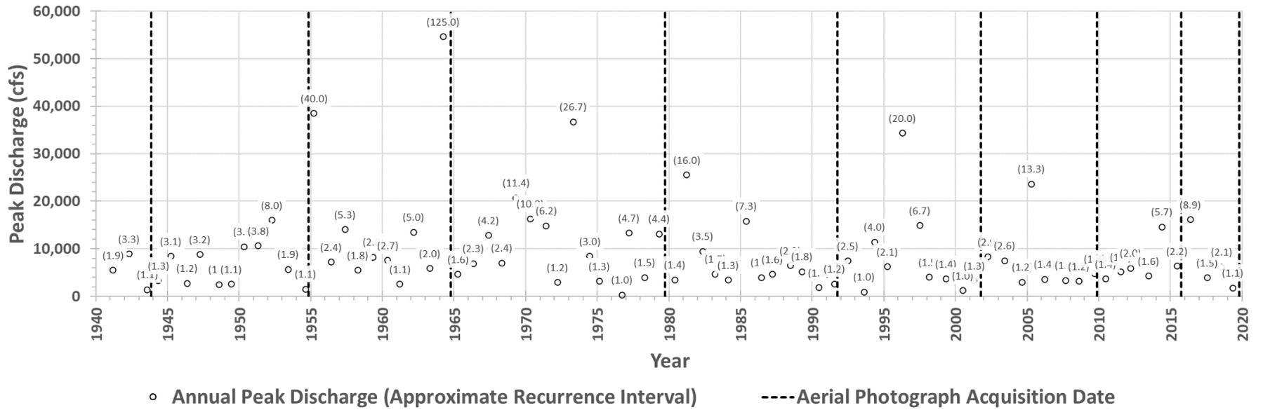
Figure 2-3. Annual peak discharge record for the Scott River (USGS gage No.11519500 near Fort Jones) associated with representative aerial photographs.
