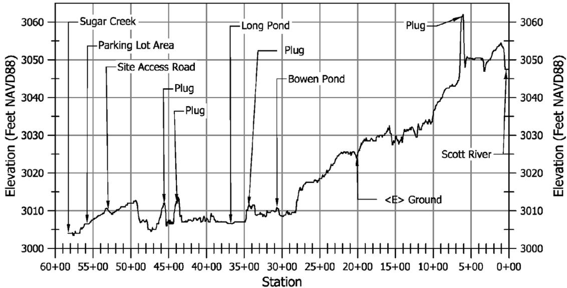
Figure 2-2. Longitudinal profile through Long Pond and adjacent ponds.
