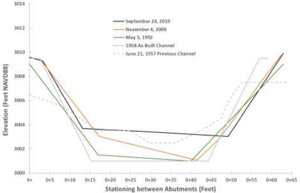
Figure H-1. Comparison of historical cross section surveys by CalTrans at the State Route 3 bridge crossing of Sugar Creek.
