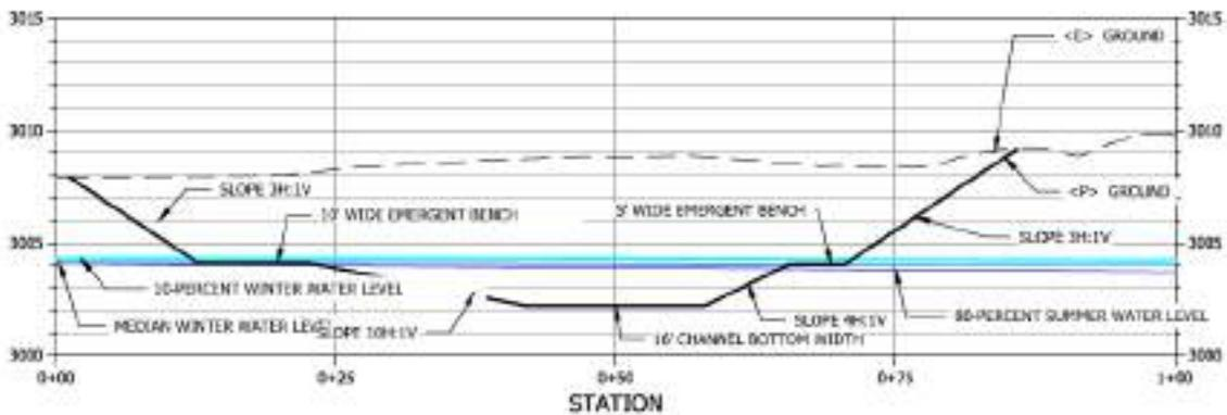
Figure 4-1. Example of typical primary connection channel cross section geometry.
