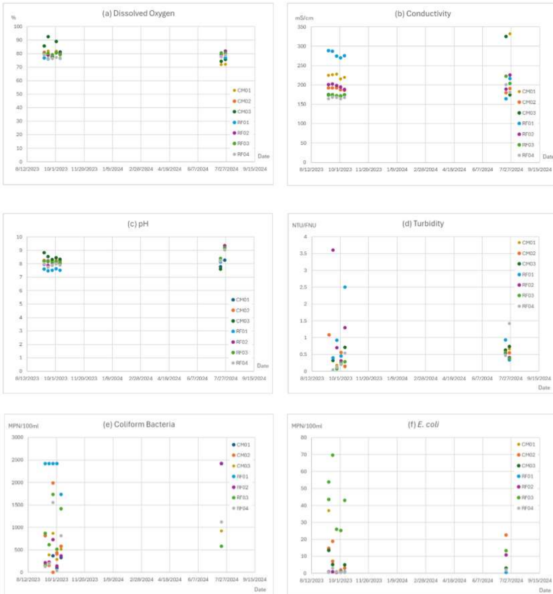
Figure 4-37. General water quality parameters for Cabin Meadow Creek and Rock Fence Creek. (a) Dissolved oxygen; (b) Conductivity; (c) pH; (d) Turbidity; (e) Coliform bacteria; (f) E. coli .
