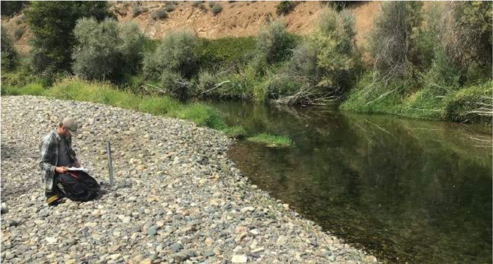
Figure 3-16. Example of Onset vented pressure transducer monitoring location SHSCMW2 on river left bar of Scott River downstream of Shackleford Creek Confluence.
